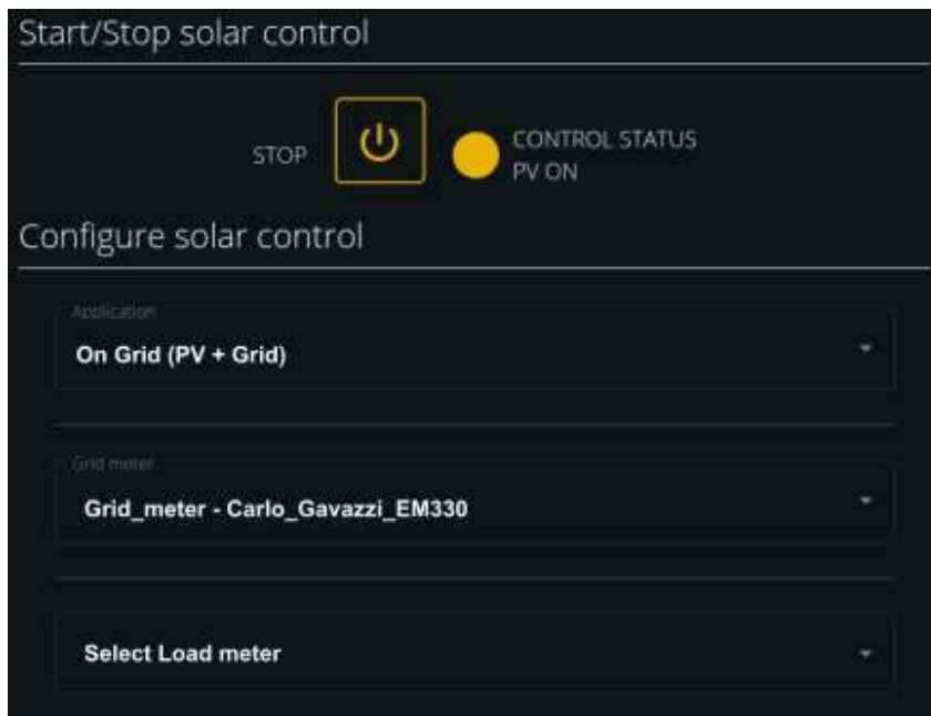
Fig. 49: eConf Control panel (PV + Grid)
