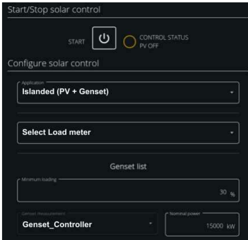
Fig. 50: eConf Control panel (PV + Genset)
